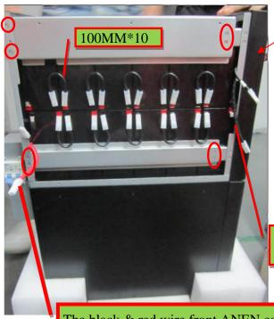
11. Screw up the Part2 & Part3 on the case by using 8 flat head screws;
