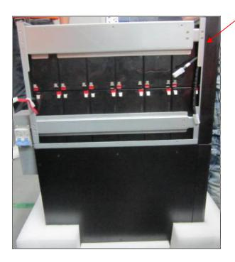
9.Put 12 batteries in the left side of the top case. (CAUTION: Keep the electrode away of the case;)
