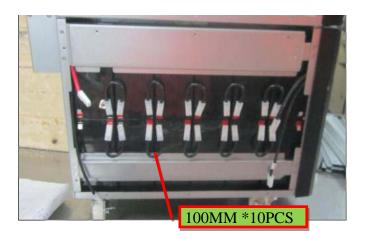
4. Connect the Batteries by 10 black wires; (Refer to the picture on the left)
